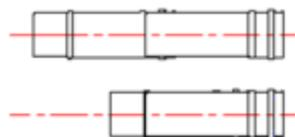
**Figure 4 – Eléments droits réglables**
